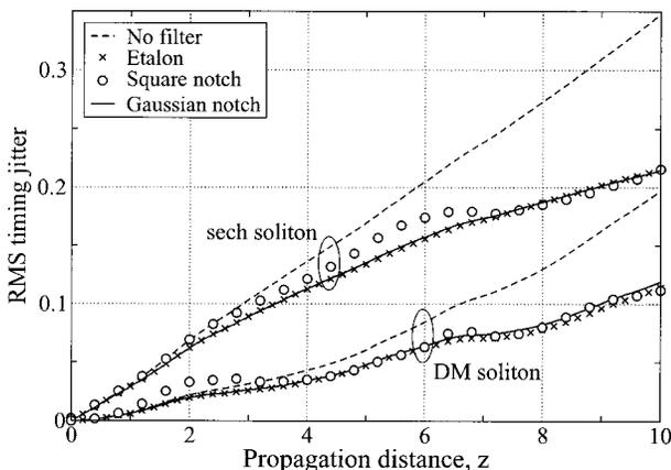
Fig. 6. Direct test of frequency-jitter suppression. The plots show the temporal offset for (a) classical solitons and (b) DM solitons versus the propagation distance. Note that although the filter effectiveness is the same for both classical and DM solitons ( $H = 4\alpha_0$ ), the frequency jitter translates to timing jitter differently for both, the DM solitons having significantly less consequent timing jitter.
