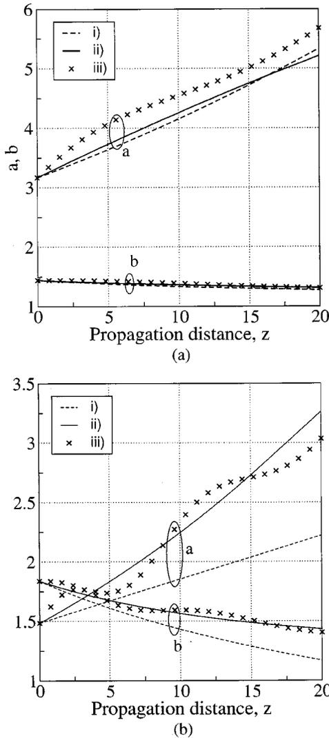
Fig. 2. Comparison between amplitude  $a$  and inverse width  $b$  of the Gaussian pulse of Eq. (8) with etalon filtering ( $\epsilon = 0.1$ ), (i) from numerical solution of the analytically derived Eqs. (14), (ii) from numerical solution of the energy-evolution Eq. (11) with  $a(E)$  and  $b(E)$  taken from numerically generated stationary DM solitons, and (iii) from direct numerical simulations of the NLSE (1).
