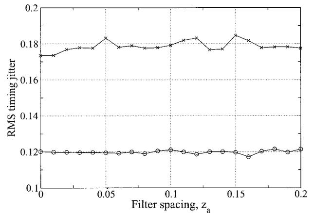
Fig. 7. Final values of the timing jitter in the lumped version of the dispersion-managed model with the Gaussian notch filters versus the normalized filter spacing  $z_a$ .
