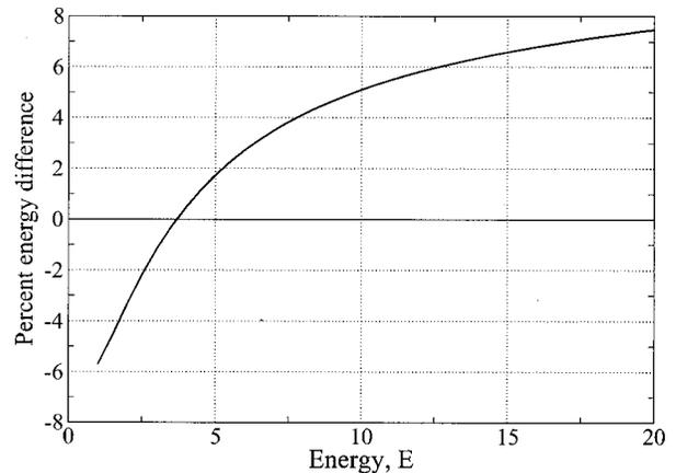
Fig. 1. Relative energy difference between a numerically exact dispersion-managed soliton (with a map strength  $S = 2$ ) and the best-fit Gaussian approximation to it, versus the net energy of the numerically found soliton.
